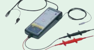
100 MHz differential probe (701921) Attenuation ratio: Can be switched between 1/10 and 1/100 Max. differential allowed voltage: ±70 V/(1/10), ±700 V/(1/100)
