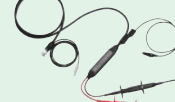
200 MHz differential probe (701922) Attenuation ratio: 1/10 with 50 Ω load Max. differential allowed voltage: ±20 V
