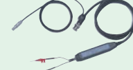
500 MHz differential probe (701920) Attenuation ratio: 1/10 with 50 Ω load Max. differential allowed voltage: ±12 V
